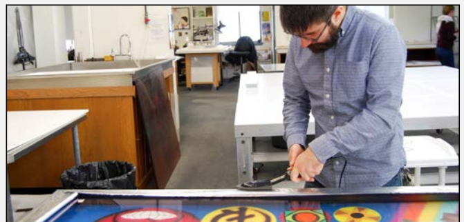
Zac Dell'Orto sealing the Marvelseal to the glazing. Image courtesy of Conservation Center for Art and Historic Artifacts.
