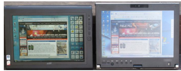
Image 2: Optically bonded display (left) versus AG air-gapped display (right)
