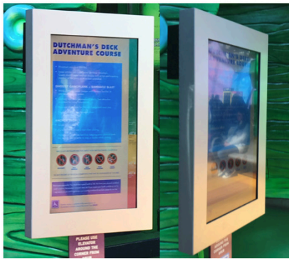
Image 1: External reflection image clarity issues (left) are exasperated when approaching display from an angle (right).
