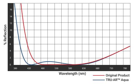
The total reflectance and transmittance of a filter depends on the type of glass used, the rear surface coating, and the combination of coatings involved: The thickness of the substrate does impact reflection.
