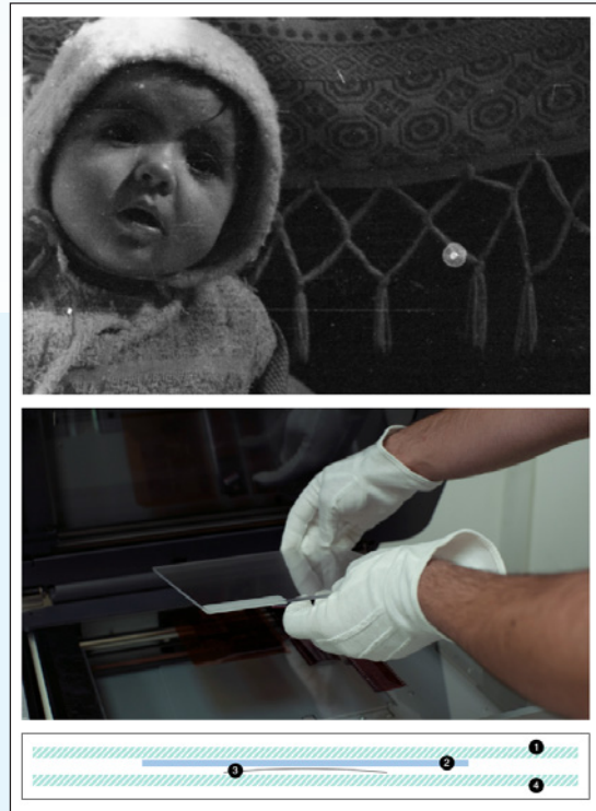
Top: Detail of the same image, scanned using the Tru Vue Reflection Control® Acrylic sheet, thus no visible Newton's rings Middle: Placing the Tru Vue Reflection Control® Acrylic over the film negatives to scan. Bottom: Ideal order of layers inside of the scanner – 1) Scanner transparency unit; 2) Tru Vue Reflection Control® Acrylic sheet; 3) Film negative, emulsion side down; 4) Scanner bed.
