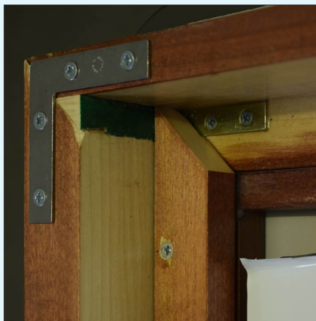
Interior view of the frame top showing the two mouldings, the triangle of wood inset to adjust for the difference, the outer L plate, part of the inner L plate, a side fillet screwed in to grip the Optium glazing (the rebating on the fillet to accommodate the L plate can just be seen) and the plastic film protecting the Optium. The glossy Dacrylate just catches the light in places.
