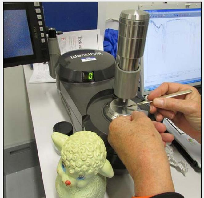
Portable FTIR machine brought into the classroom at "Masterclass in Plastics" to use for plastic identification purposes.
