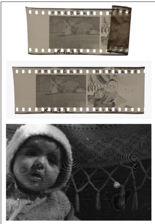
Top: Scan of a nitrate film negative, placed as it is on the scanner bed. Middle: Scan of the same film negative, held down to the scanner bed using a clear glass sheet. Bottom: Detail of the image exhibiting Newton's rings while using the glass sheet.
