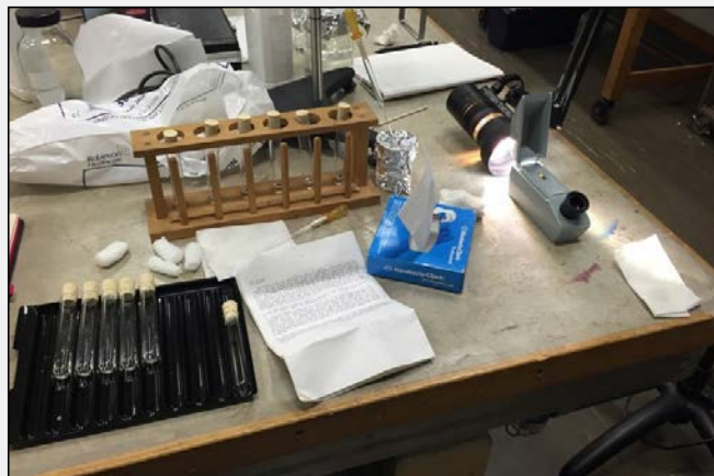
Testing different mixtures of mineral solvents and clove oil for their refractive index. We could then replicate an adhesive with a certain RI on a crack in a piece of glass (Melissa Lewis).
