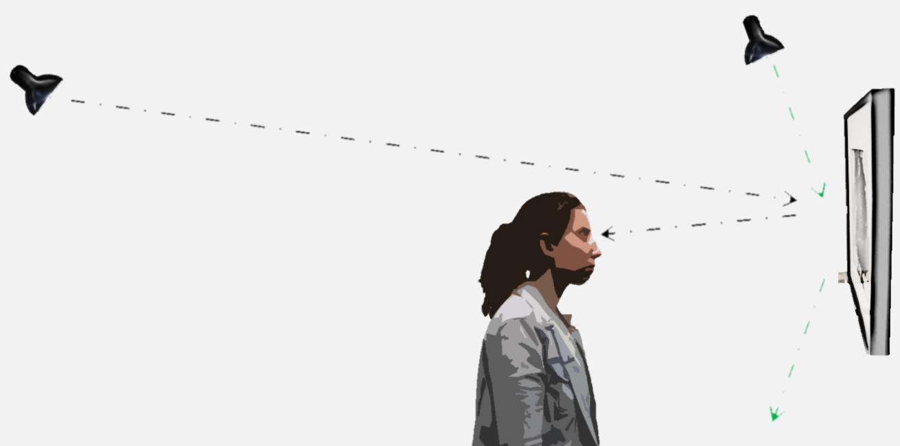
Fig. 8 In an ideal world light sources would be placed at a high, sharp angle to a work, causing any residual reflections to be directed towards the ground. In reality, many exhibition spaces have light from multiple directions including across the room. These can cause reflections at eye level.
