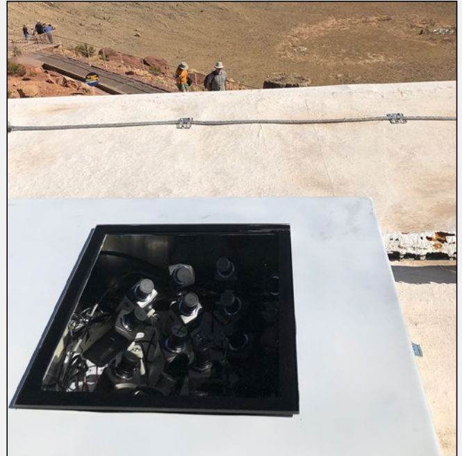
Tru Vue® UltraVue® Laminated Glass protects the newly installed fireball camera station’s 16 mounted cameras. Photo courtesy of Dr. Nick Moskowitz, Lowell Observatory.
