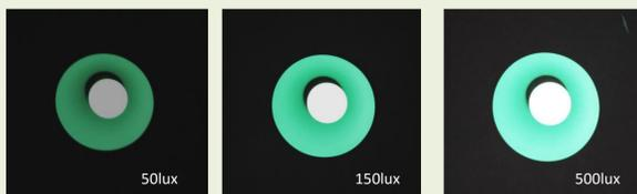
Fig. 4 Reflection of 4000K LED seen in Optium Museum Acrylic with black background at varying illuminance measured with Sunche Professional Illuminance Meter
